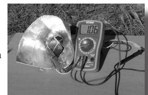
*Solar cell (bottom of funnel) attached to meter.*
